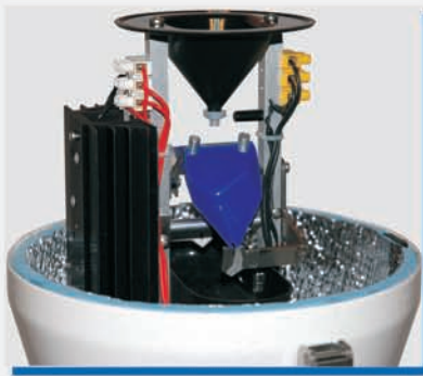
Measuring mechanism of rain gauge
